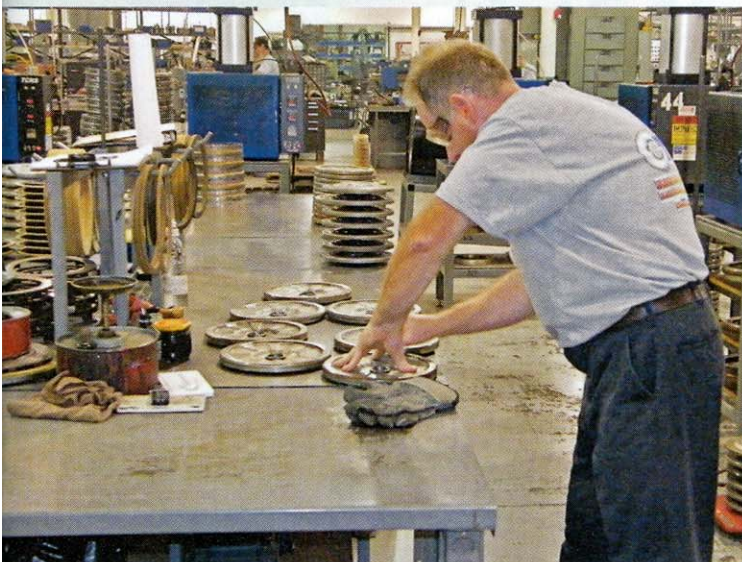
In the critical bonding subassembly work area, torque-converter pistons are prepared to receive new friction material.
