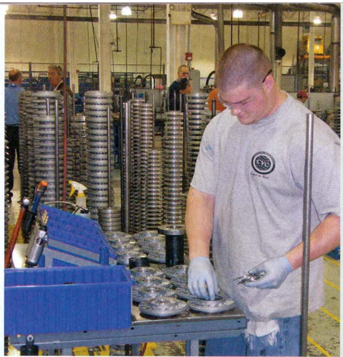
A separate subassembly area is devoted to preparing stators for the final-assembly stations.
