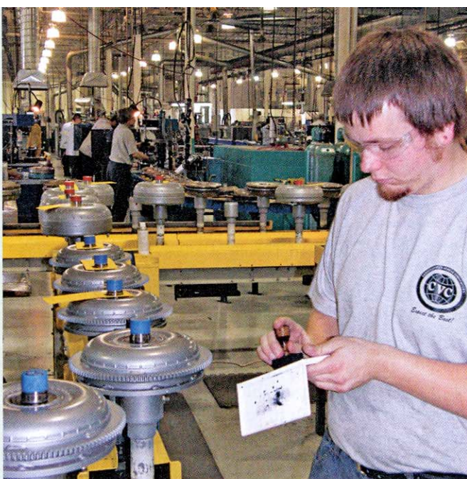
Approaching the end of the assembly line, assembled converters receive a coat of paint and are labeled for entry into the inventory system.
