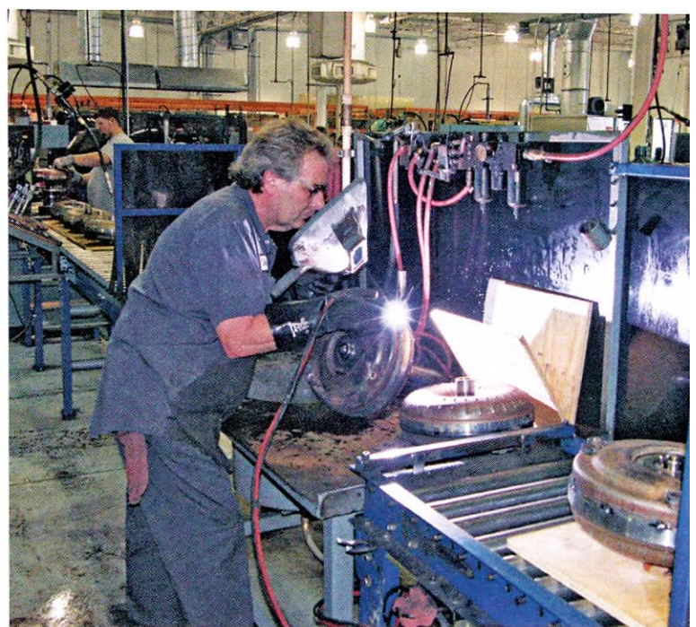
On the final-assembly line, the converter outer body is welded.
