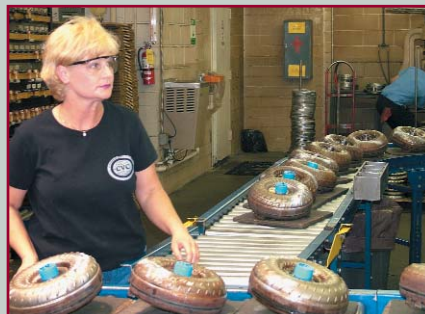
Marcia Maynard-Prugh is capping converters after they have been leak-tested and balanced.
