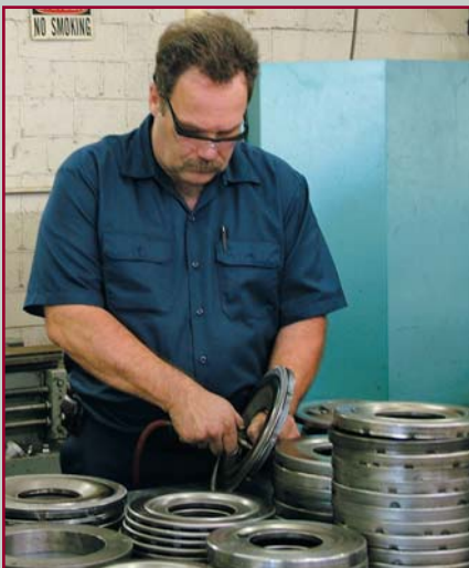
Pistons are processed and prepared before the crucial bonding step.
