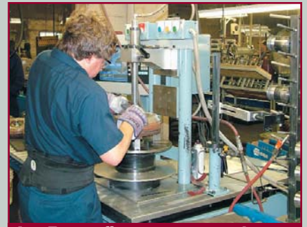
Joe Foster first came to work at MAMCO in 1974. He gives a final yes or no as CVC converters are tested on the high-tech balancing equipment.
