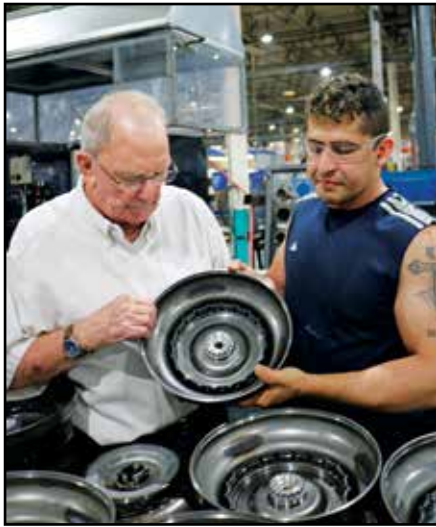
John Maynard (right) inspecting front covers for Mercedes 722.6/722.9 applications. These units will have the front cover hubs and seals replaced before being used for assembly into remanufactured converters.
