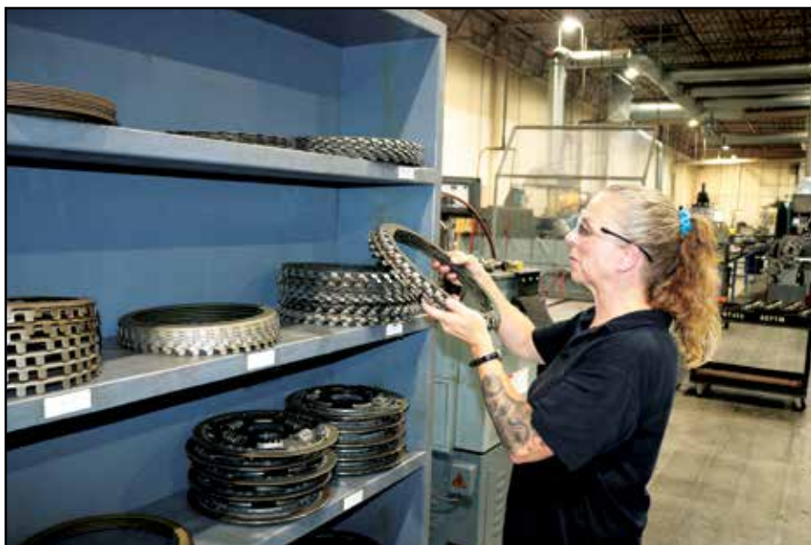
New captive clutch friction plates are used in the 6R80 remanufacture.
