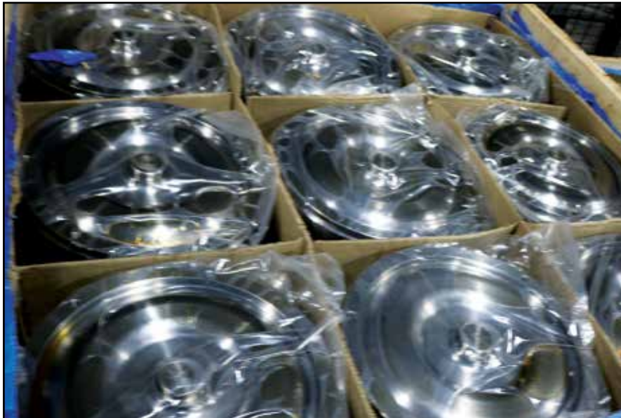
One-piece billet covers have been inspected, cleaned and are now ready to be placed on the assembly line.
